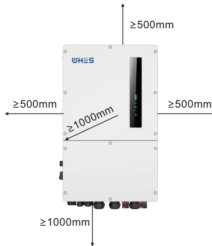
Figure 3.5 Inverter Mounting Clearances
