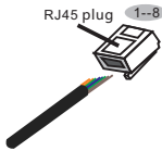
Figure 3.21 Strip the insulation layer and connect to RJ45 plug
